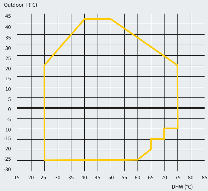
OPERATING LIMITS IN DOMESTIC HOT WATER
